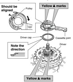
2. Secure the cassette joint to the hub with the cassette joint fixing ring. When installing the cassette joint fixing ring, align the yellow ● mark with the yellow ● mark on the cassette joint pulley, and then turn the cassette joint fixina rina 45° clockwise.
