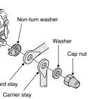
5. Fix the brake arm of the Inter-M brake securely to the chainstay with the brake arm clip.
